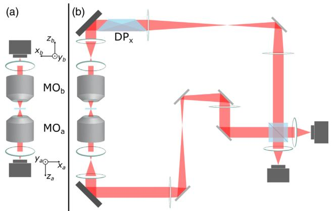
FIG. 3. Dual-objective collection schematics. (a) Signals collected by microscope objectives  $a$  and  $b$  ( $\text{MO}_a, \text{MO}_b$ ) detected on two cameras without recombination. (b) Interferometric detection. Optimal lateral localization requires an additional reflection in one arm, enforced here by an  $x$ -oriented Dove prism ( $\text{DP}_x$ ).
