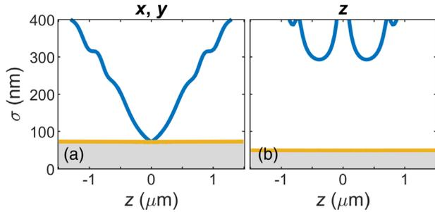
FIG. 4. Photon-normalized precision bounds for dual-objective collection. For  $N$  detected photons, divide the vertical axis by  $\sqrt{N}$ . (a) Lateral localization bounds. The gray shaded region is bounded above by  $\sigma = \sigma_x^{(\text{QCRB})} = \sigma_y^{(\text{QCRB})}$ . Blue curve:  $\sigma_{x,y}^{(\text{CRB})}$  for non-interferometric detection. Gold line: interferometric detection. (b) Depth localization bounds. The color code corresponds to that in (a).
