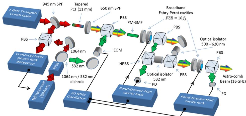
Fig. 2 Schematic of green astro-comb setup.
