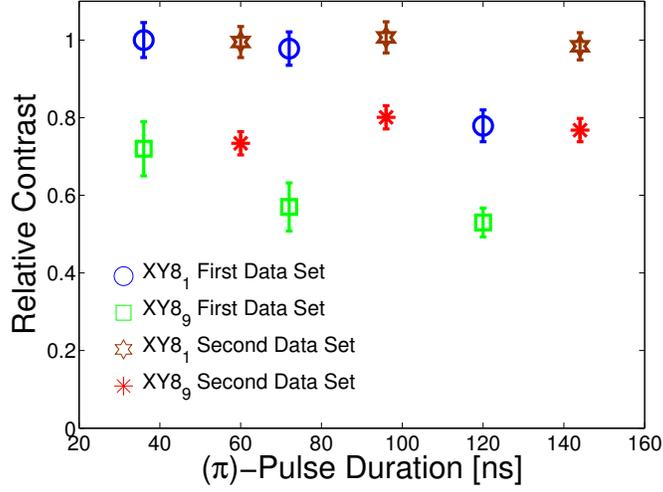
Figure S7: Relative contrast in the decoherence-free limit ( $\tau \ll \frac{T_2}{n}$ ) as a function of ( $\pi$ )-pulse duration for two experimental configurations: the first one with the hyperfine structure shown in Fig. 1(c) of the main text, the second one with the hyperfine structure shown in Fig. S5. The results are shown for  $XY8_1$  (8 pulses) and  $XY8_9$  (72 pulses).
