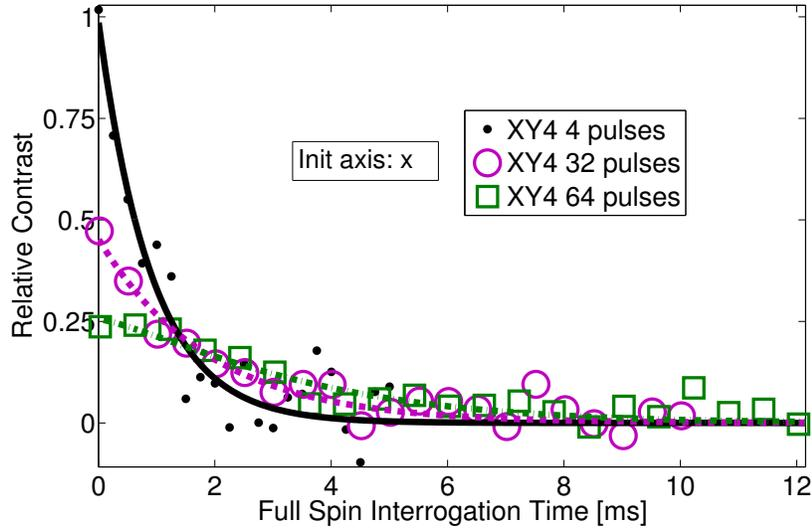
Figure S3: Full coherence curves along the x axis for the XY4 sequence, at 4 (black, solid lines), 32 (purple, dashed lines) and 64 (green, dash-dotted lines) pulses.
