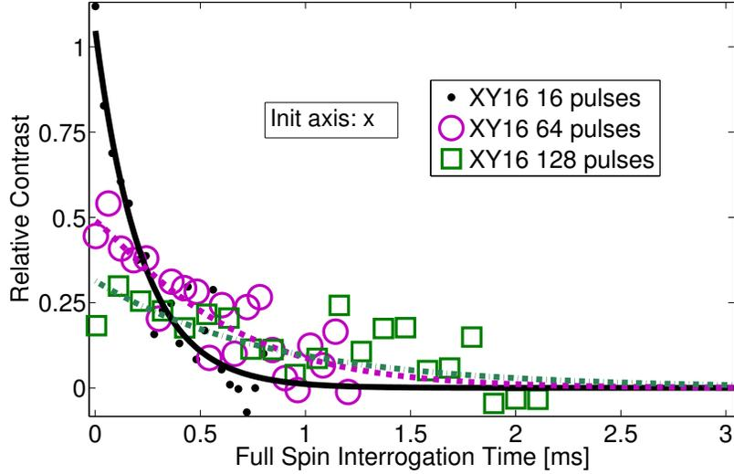
Figure S4: Full coherence curves along the x axis for the XY16 sequence, at 16 (black, solid lines), 64 (purple, dashed lines) and 128 (green, dash-dotted lines) pulses.
