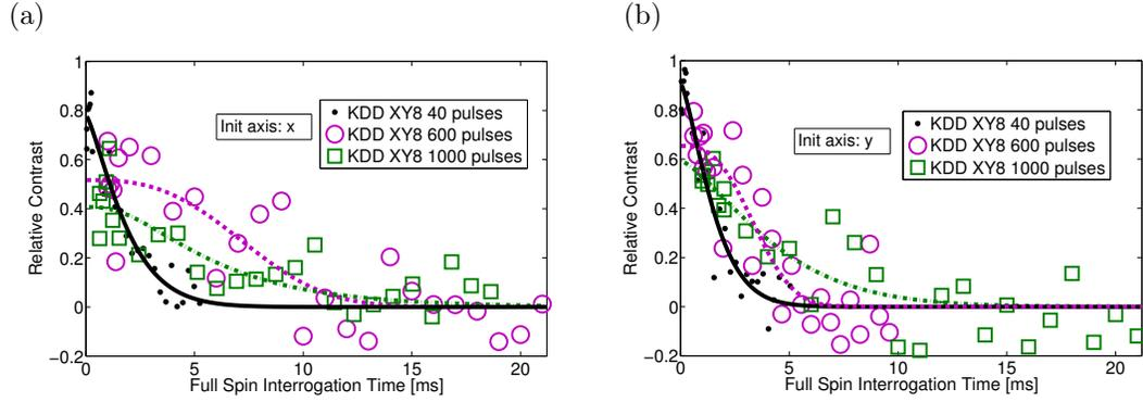
Figure S2: Full coherence curves for the KDD XY8 sequence, at 40 (black, solid lines), 600 (purple, dashed lines) and 1000 (green, dash-dotted lines) pulses. (a) initialization along the x axis (b) initialization along the y axis.
