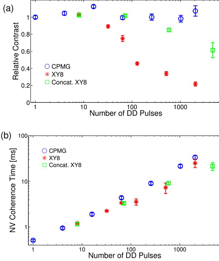
Figure S6: (a) Relative contrast in the decoherence-free limit ( $\tau \ll \frac{T_2}{n}$ ) of DD protocols as a function of number of pulses for the second data set. (b) The coherence time of DD sequences as a function of the number of pulses for the second data set.
