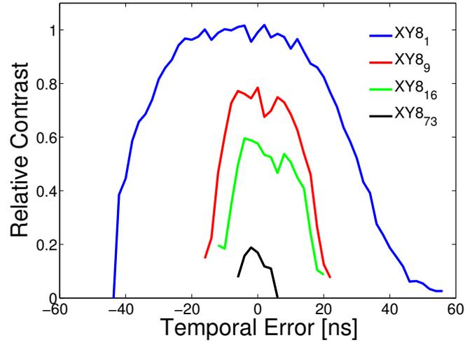
Figure S8: Relative contrast in the decoherence-free limit ( $\tau \ll \frac{T_2}{n}$ ) as a function of temporal deviation from a correct ( $\pi$ )-pulse. The results are shown for  $XY8_1$  (8 pulses),  $XY8_9$  (72 pulses),  $XY8_{16}$  (128 pulses) and  $XY8_{73}$  (584 pulses).
