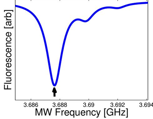
Figure S5: Optically detected magnetic resonance measurement of  $|0\rangle \leftrightarrow |+1\rangle$  transition in an NV ensemble, with better alignment of a static  $\sim 300$  G magnetic field, creating higher polarization of the  $^{14}\text{N}$  nuclear spins into the  $|-1\rangle$  spin state.
