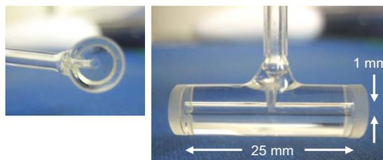
FIG. 1. (Color online) Photographs of the narrow (1 mm) paraffin-coated <sup>87</sup>Rb vapor cell (see text).
