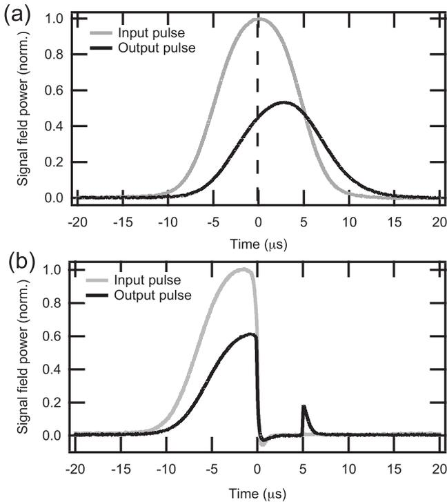
FIG. 3. (a) Measured slow light in the narrow coated cell with shorter coherence time. Fractional delay is 0.26 and transmission fraction is 0.53.  $T=60$  °C and  $I=250$  mW/cm<sup>2</sup>. The transmission for the cell with longer coherence time, at the same fractional delay, is only 0.40. (b) Stored light under the same conditions, with a 5  $\mu$ s storage time.
