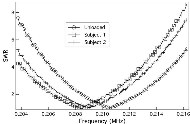
**Fig. 8.** Measured SWR as a function of frequency for the human chest coil unloaded as well as loaded by two different human subjects weighing between 60 and 80 kg.
