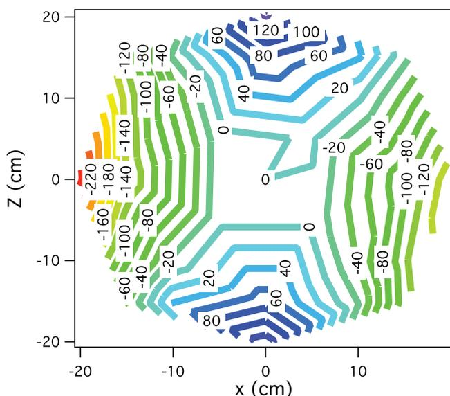
**Fig. 4.**  $B_0$  field map for the  $x$ - $z$  plane, obtained after optimization of passive shim placement. Contours indicate deviation of <sup>1</sup>H NMR frequency in Hz from the zero-center frequency of 210 kHz. Across a human lung of width  $\sim 25$  cm,  $\nu_0 \sim \pm 80$  Hz, which implies the  $B_0$  homogeneity  $\Delta B_0 \sim \pm 0.02$  G or about 350 ppm.
