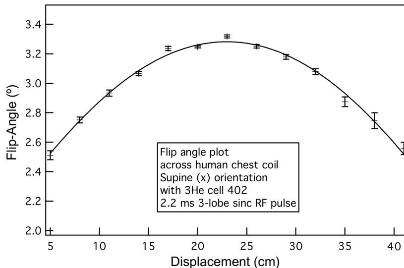
**Fig. 7.** Measured <sup>3</sup>He flip-angle versus position along the center axis of the human chest coil oriented for supine lung imaging (i.e., along the imager's *x* axis). Flip-angle calibrations were performed on hyperpolarized <sup>3</sup>He cell #402 which had a 3 cm width along the *x* axis. Displacement is measured from one end of the chest coil. The solid curve is a fit of the data to the function describing the *B<sub>1</sub>* field created by an ideal finite solenoid.
