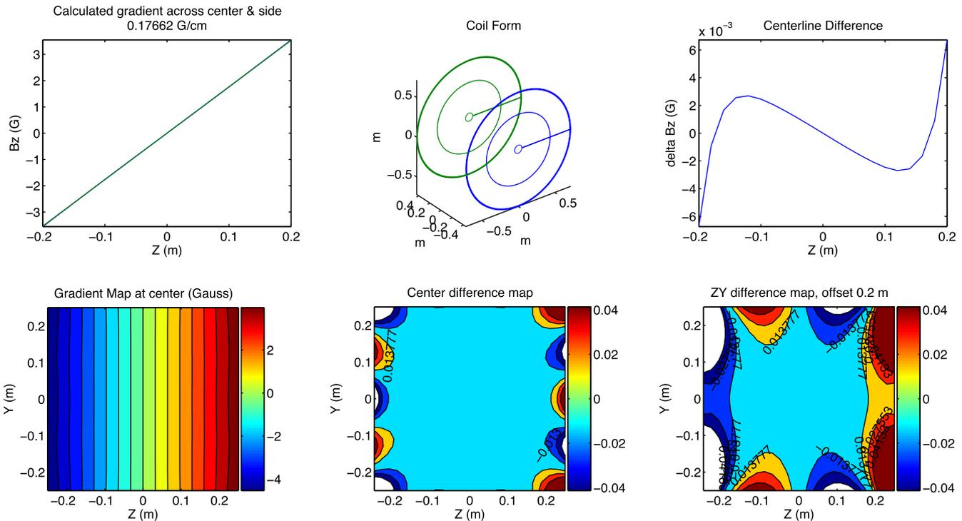
**Fig. 5.** Sample output of the MATLAB gradient coil optimization routine, in this case for a  $z$  gradient coil form. The program determines the magnetic field strength and produces a predicted gradient field map as well as plots of the deviation from an ideal gradient for the given coil design under consideration.
