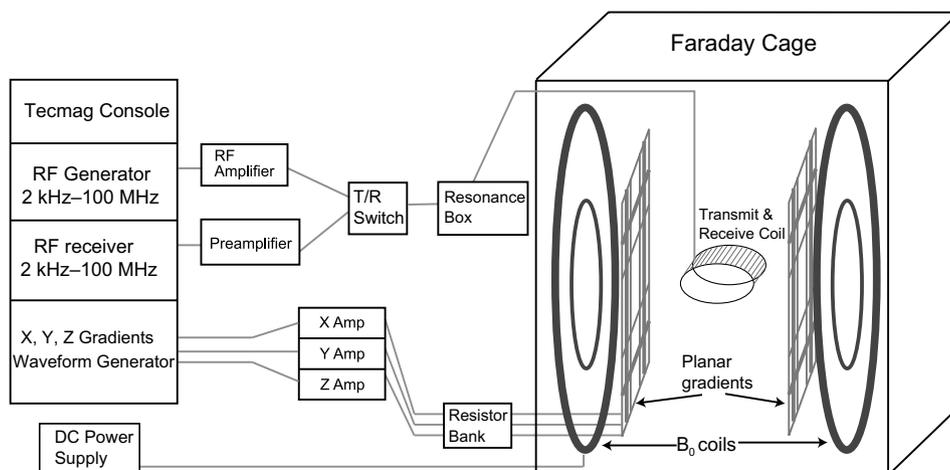
**Fig. 1.** Schematic of the open-access human MRI system. The major components include an MRI research console (left), electronics components for RF and gradient pulse generation and  $B_0$  control (center), and the  $B_0$ , gradient and  $B_1$  coils, located inside an RF-shielding Faraday cage (right). The resonance box, T/R switch and preamplifier are located inside the Faraday cage, but are drawn as shown for clarity.
