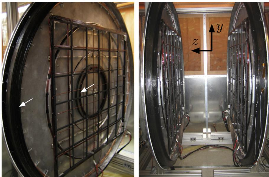
**Fig. 2.** Left: The  $B_0$  and gradient coils mounted on the aluminum flange. The arrows point to the outer and inner  $B_0$  coils. The other circular coils are the  $z$  gradient coils, while the rectangular coils are the  $x$  and  $y$  gradient coils. Right: A view of the imaging region with the imaging axes defined. The  $x$  axis points out of the page.
