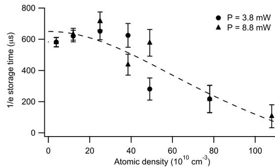
**Figure 4.** Lifetimes of stored coherence as a function of atomic density, derived from measurements described in text. The coherence lifetime drops at high atomic density, likely due to the effect of temperature-dependent losses such as Rb-Rb spin exchange. Error bars are derived from Rb temperature and laser frequency uncertainty as well as statistical uncertainty in fits to coherence lifetimes. *Dashed line added to guide the eye.*
