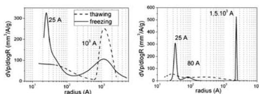
Fig. 2 Capacitive method: freezing and thawing of cement paste at 1 (left) and 7 (right) days.
