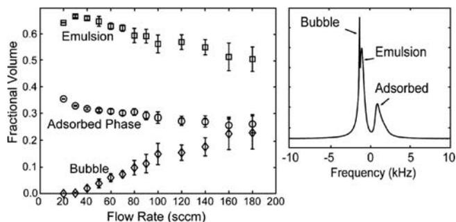
Fig. 1 Fractional volumes of <sup>129</sup>Xe within the bubble, emulsion and adsorbed phases of the Al<sub>2</sub>O<sub>3</sub> particle bed as a function of flow rate. Each point is the average of 32 separate single-shot spectra acquired over a 5-min period. An example <sup>129</sup>Xe gas spectrum acquired from the Al<sub>2</sub>O<sub>3</sub> bed at a flow rate of 50 standard cm<sup>3</sup>/min is shown in the inset.
