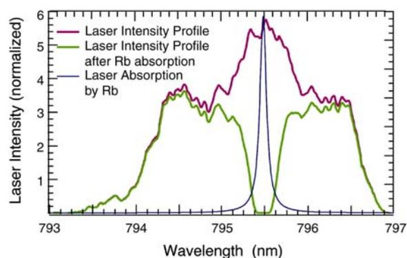
Fig. 1 Laser line-shape from a typical LDA commonly used for spin-exchange optical pumping. The pink line is the measured laser output, the green line is the laser spectrum after travelling through an optical pumping cell. The blue line is the calculated laser absorption by rubidium in the spin-exchange process, for common <sup>129</sup>Xe operating parameters.
