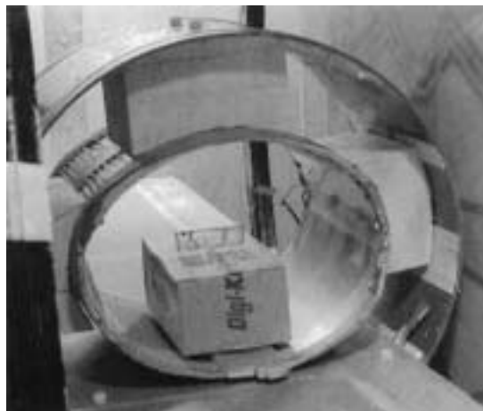
Figure 6 Photograph of the transmit and receive coils for the open-access human MRI system. The large Helmholtz transmit coil was bolted onto the subject imaging table, and the receive coil was attached using foam spacers and plastic bolts.
