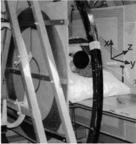
Figure 5 The planar gradient sets mounted on the aluminum support frame of the open-access human MRI B_0 coil system. The x and y gradients are placed just inside of the z gradients, relative to the subject (seen in supine position). As such the z -axis gradient is visible on the subject's left, and the x -axis gradient is seen to his right.
