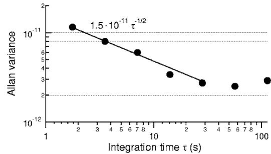
Fig. 4. Measured frequency stability of a 100 MHz crystal oscillator locked to the  $^{87}\text{Rb}$   $N$ -resonance, relative to a hydrogen maser. The solid line is a fit to the early time measurements.
