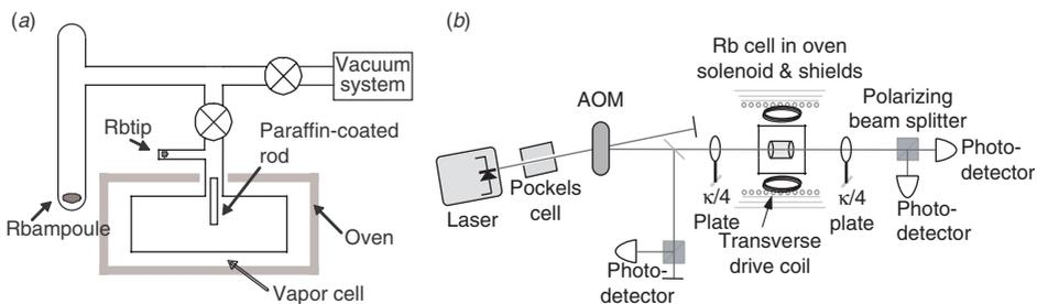
Figure 1. (a) Schematic of the Pyrex manifold and vacuum system used to apply paraffin coating to the inside of the cell. (b) Schematic of the apparatus for double resonance, EIT, and slow light experiments. See text.
