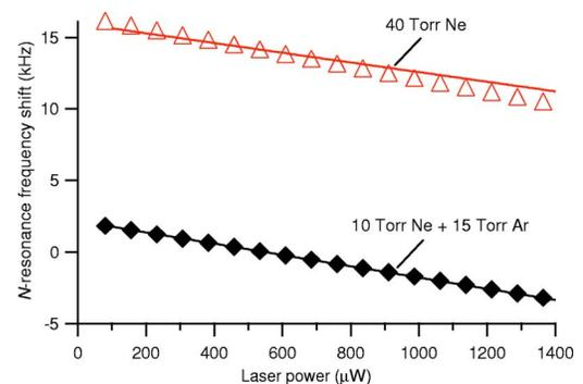
FIG. 6. (Color online) Measured dependence of the  $N$ -resonance frequency on the total incident laser power, with the probe field tuned  $\approx 300$  MHz below the  $F=2 \rightarrow F'=2$  transition of  $^{87}\text{Rb}$ . Upper trace: 40-Torr Ne ( $\Delta$ ). Lower trace: 25-Torr Ne-Ar mixture ( $\blacklozenge$ ). As in Fig. 5, the  $N$ -resonance frequencies include the buffer gas pressure shift. The solid lines are calculations from an analytical model.
