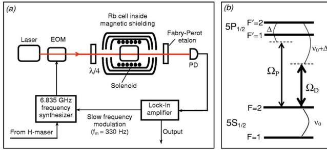
FIG. 2. (Color online) (a) Experimental apparatus. (b) Energy levels and applied fields ( $\Omega_p, \Omega_D$ ) for  $N$  resonances on the  $D_1$  line of  $^{87}\text{Rb}$ .  $\nu_0$  is the ground electronic state hyperfine splitting and  $\Delta$  is the detuning of the probe field from the  $F=2 \rightarrow F'=2$  transition.
