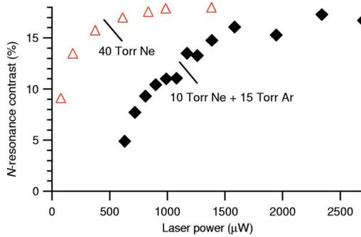
FIG. 4. (Color online) Measured dependence of  $N$ -resonance contrast on the total incident laser power for two buffer gas cells: 40-Torr Ne ( $\Delta$ ) and 10-Torr Ne + 15-Torr Ar ( $\blacklozenge$ ). The probe field is tuned  $\approx 300$  MHz below the  $F=2 \rightarrow F'=2$  transition of  $^{87}\text{Rb}$ .
