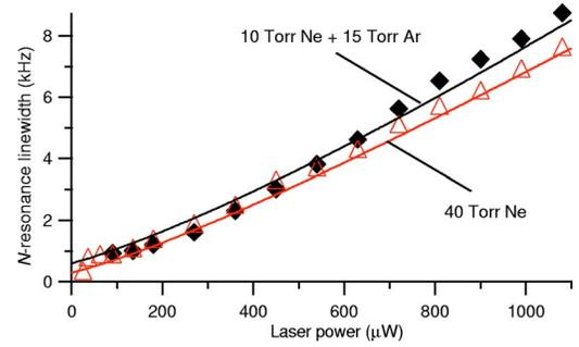
FIG. 3. (Color online) Measured  $N$ -resonance linewidth as a function of total incident laser power for  $^{87}\text{Rb}$  vapor cells filled with 40 Torr of Ne buffer gas ( $\Delta$ ) and a mixture of 10-Torr Ne and 15-Torr Ar ( $\blacklozenge$ ). The probe field is tuned  $\approx 300$  MHz below the  $F=2 \rightarrow F'=2$  transition of  $^{87}\text{Rb}$ . The solid lines are calculated linewidths using an analytical  $N$ -resonance model.
