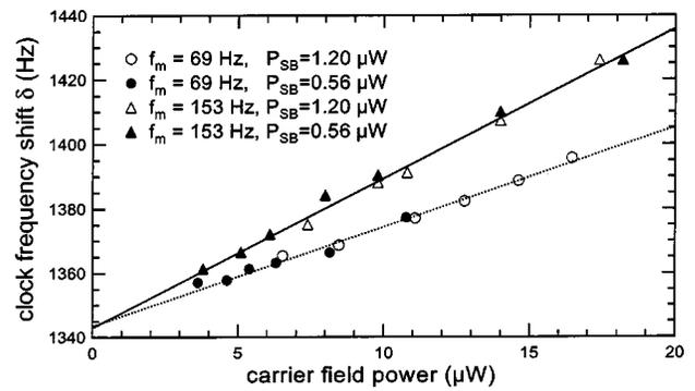
Fig. 5. Measured dependence of the CPT clock frequency on carrier field power at one-photon resonance ( $\Delta = 0$ ), for two slow-phase-modulation frequencies and two total powers in the first-order sidebands. (Uncertainties in the measured clock frequencies are approximately equal to the size of the points.) Linear fits are shown for all data points at each of the two modulation frequencies.
