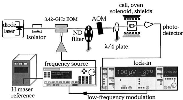
Fig. 2. Schematic of the apparatus.
