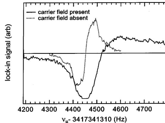
Fig. 6. CPT resonances with (solid curve) and without (dotted curve) the carrier field present. Both data sets were taken with  $f_m = 98$  Hz and  $\epsilon \approx 0.6$  and with a vapor cell containing isotopically enriched <sup>87</sup>Rb and 22 Torr of Ne buffer gas.<sup>15</sup>
