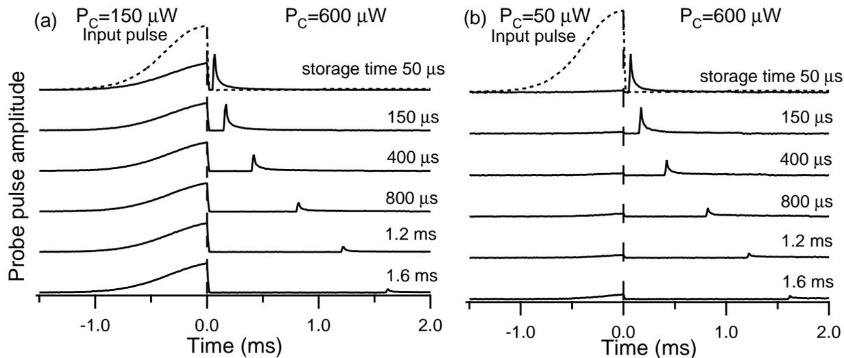
**Figure 4.** Light storage for various storage intervals and two control field powers during the write process: (a)  $150 \mu\text{W}$  and (b)  $50 \mu\text{W}$ . The input pulse duration (dashed line) is  $500 \mu\text{s}$  and the retrieve control power is  $600 \mu\text{W}$  for all measurements. Variations in the amplitude of the leading (slow light) pulse are due to drifts of the laser frequency, which affects the group velocity of the probe pulses.
