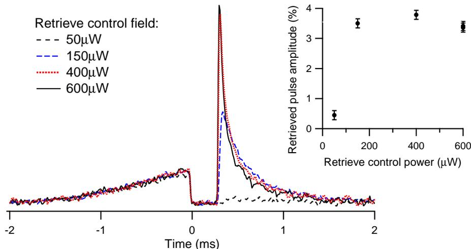
**Figure 6.** Retrieved pulse at several retrieve control field intensities. The storage time is  $300 \mu\text{s}$  and the intensity of the control field during the writing stage is  $50 \mu\text{W}$ . *Inset:* the retrieved probe pulse area normalized to the input pulse area as a function of the retrieve control field.
