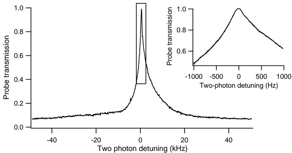
**Figure 8.** Probe transmission as a function of two photon detuning (*i.e.*, EOM drive frequency). *Inset:* Central region of the resonance. ( $P_c \approx 150 \mu\text{W}$ .) The amplitude of the peak is normalized to the maximum transmission under EIT conditions. Some asymmetry of the resonances is due to drift of the laser from the atomic resonance.
