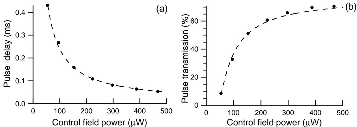
**Figure 3.** (a) Delay of the probe pulse propagating through the Rb cell under slow light conditions as a function of the control field power  $P_c$ ; the dashed line is the best fit of the experimental points given by Eq. (1). (b) Transmitted amplitude of the probe pulse versus control field power; the dashed line is the best fit of the experimental points given by Eq. (2). The probe pulse has a Gaussian form with a FWHM  $\approx 1$  ms.
