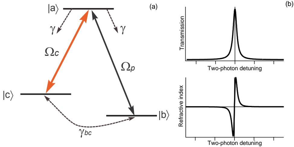
**Figure 1.** (a) Idealized interaction scheme for the control field  $\Omega_c$  and probe field  $\Omega_p$  with three-level atoms in  $\Lambda$  configuration. (b) Transmission and dispersion lineshapes for EIT in a three-level system.
