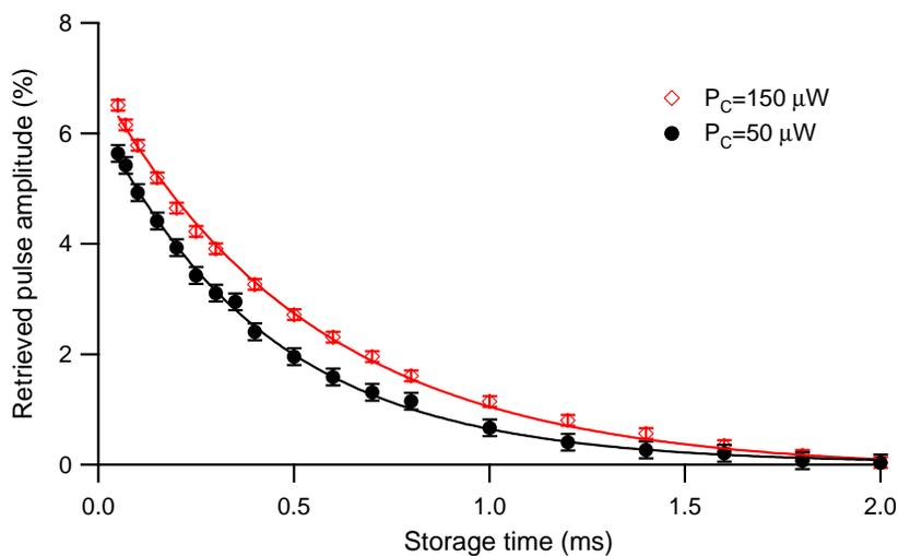
**Figure 5.** The ratio of the retrieved probe pulse area to the input pulse area (the efficiency as defined in the text) as a function of the storage time for two different write control fields:  $50 \mu\text{W}$  ( $\bullet$ ) and  $150 \mu\text{W}$  ( $\diamond$ ). The  $1/e$  decay times from exponential fits (solid lines) are respectively  $430 \mu\text{s}$  and  $550 \mu\text{s}$ .
