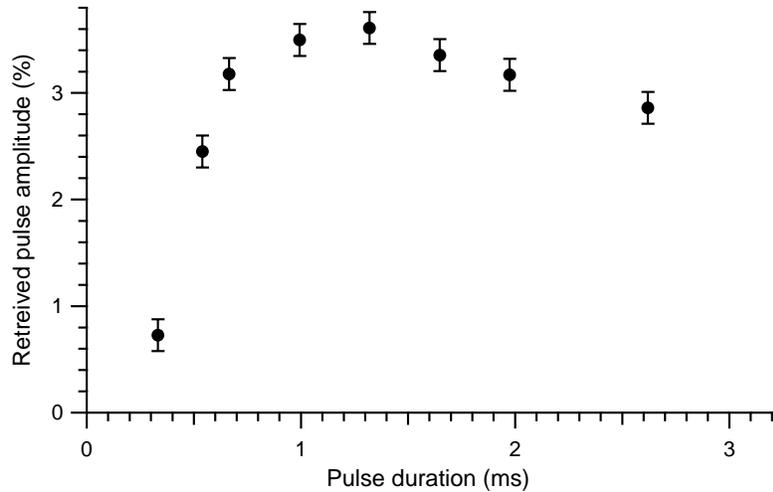
**Figure 10.** Retrieved pulse area normalized to input pulse area as a function of pulse duration. The control field power ( $P_c$ ) during the writing stage is  $50 \mu\text{W}$ , and is  $600 \mu\text{W}$  during the retrieval stage. The storage time is  $100 \mu\text{s}$ .
