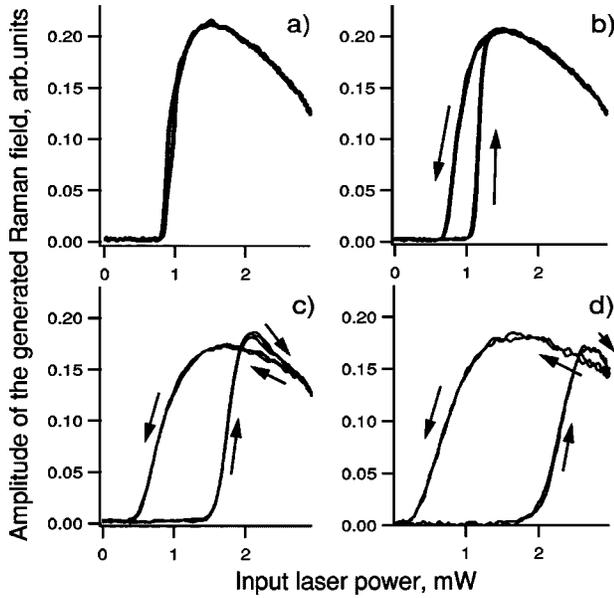
FIG. 3. Differing degrees of observed hysteresis in the generated Raman Stokes field  $E_1$  as the corresponding  $\Omega_1$  pump field intensity is modulated at (a) 10 Hz (no hysteresis); (b) 150 Hz; (c) 1.2 kHz; (d) 4 kHz. Several (two to three) cycles are shown on each plot to demonstrate the reproducibility of the data, with arrows indicating the “direction” of change of the pump field. The off-resonant laser detuning  $\Delta$  was approximately 4 GHz.
