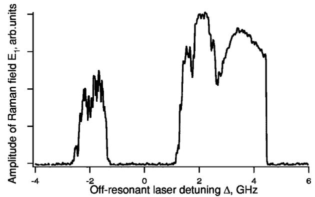
FIG. 2. Example spectrum of the generated Raman Stokes field  $E_1$  as a function of the detuning  $\Delta$  of the off-resonant pump field  $\Omega_1$ .
