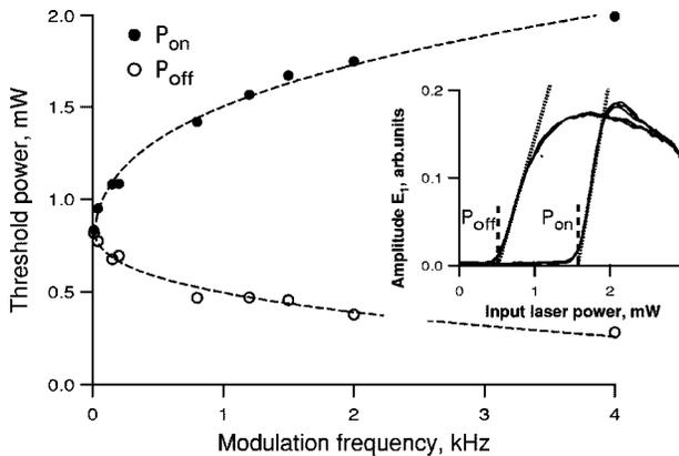
FIG. 4. Measured dependence on modulation frequency of the hysteresis threshold powers,  $P_{\text{on}}$  and  $P_{\text{off}}$ , of the off-resonant pump field. The dashed lines indicate independent fits of  $P_{\text{on}}$  and  $P_{\text{off}}$  to  $\sqrt{f_{\text{mod}}}$ . Inset: Graphic definition of the manner in which  $P_{\text{on}}$  and  $P_{\text{off}}$  were determined from the hysteresis data.
