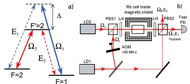
FIG. 1. (a) Three-level double- $\Lambda$  scheme used in the experiment. The first diode laser LD1 (pump field  $\Omega_1$ ) is detuned by  $\Delta \approx 4$  GHz to the blue side of the Rb transition  $F=1 \rightarrow F'=2$ . The second laser LD2 (pump field  $\Omega_2$ ) is resonant with  $F=2 \rightarrow F'=2$ . (b) Experimental setup.
