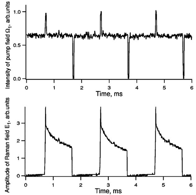
FIG. 5. Demonstration of an all-optical switch using dynamic optical bistability. The Stokes field  $E_1$  could be switched on and off (lower graph) by pulsing the pump field  $\Omega_1$  (top graph). The duration of the  $\Omega_1$  pulses was 40  $\mu\text{s}$ ; the plotted intensity of these pulses is normalized to their maximum value ( $\approx 2.5$  mW) with a detuning  $\Delta \approx 4$  GHz.
