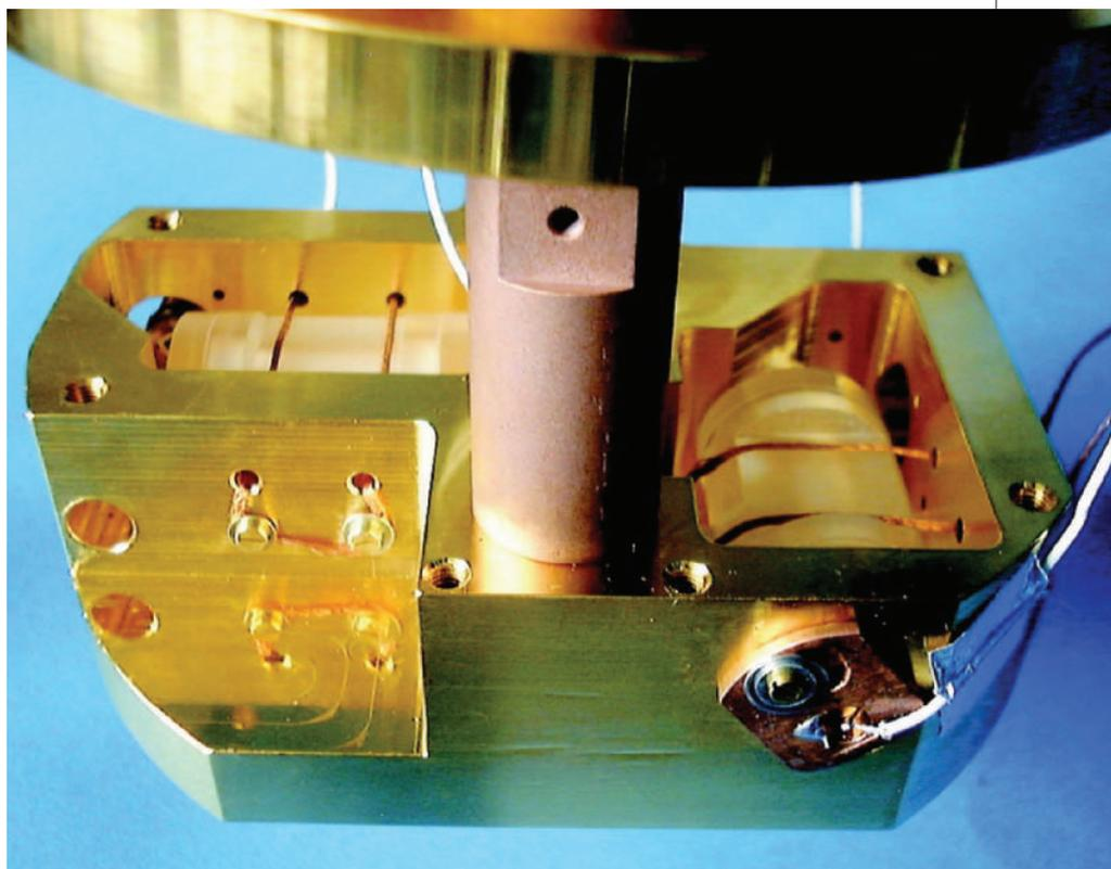
**Light box:** Michelson and Morley's original experimental set-up (right) and its modern-day equivalent (above) — optical resonators that measure the speed of light more accurately.
