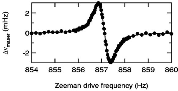
FIG. 2. A double resonance measurement of the Zeeman frequency ( $\nu_Z$ ) in the H maser. The change from the unperturbed maser clock frequency is plotted versus the driving field frequency. (The statistical uncertainty in each point is approximately  $50 \mu\text{Hz}$ .) The solid line is the fit of an antisymmetric line shape [16] to the data, yielding  $\nu_Z = 857.125 \pm 0.003 \text{ Hz}$  in this example.
