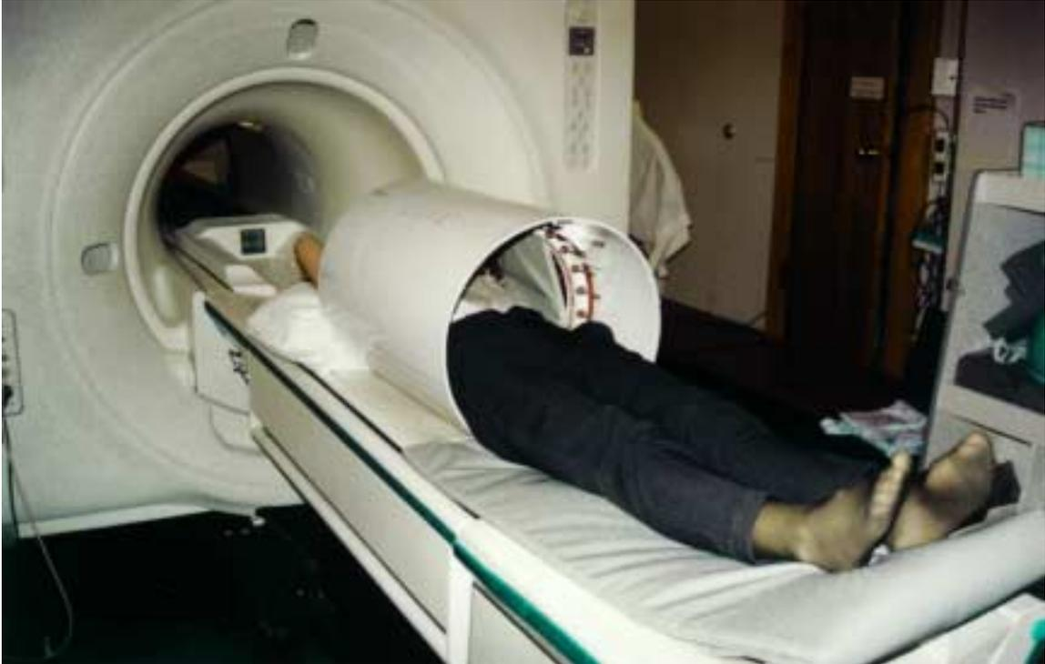
Figure 8. Photograph of the GE-ANMR 3 T full body system with subject positioned in volume chest coil
