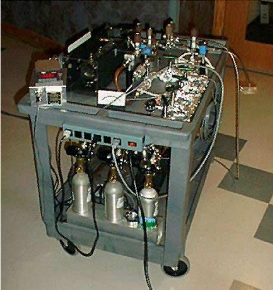
Figure III.1. Front of human inhalation cart. Xe, N<sub>2</sub>, and He cylinders are visible, as are the temperature and pressure gauges. The oven surrounding the pump cell (black casing on left side of cart) has been opened to provide a view of the pump cell. A small inhalation bag mated to the cart outlet is visible on the right side.
