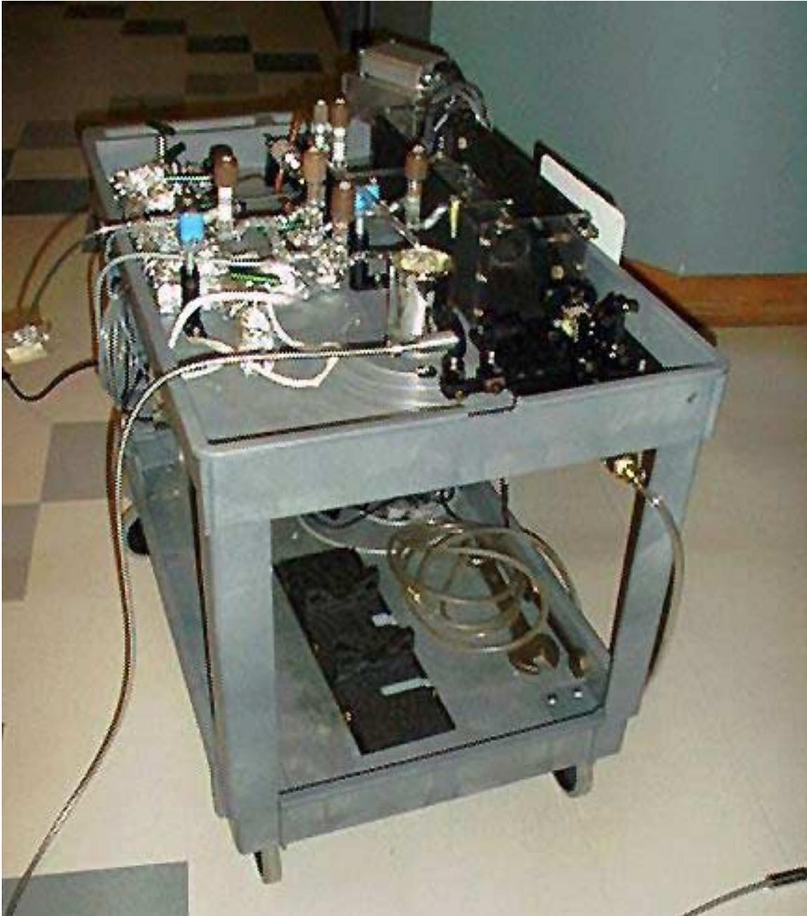
Figure III.2. Back of human inhalation cart. The fiber glass cable from the laser diode arrays is visible, as are the laser-guiding and polarizing optics.
